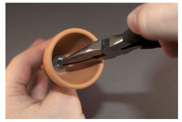
Once the threading is started, finish by securing the screw eye with a pair of needle-nose pliers. (Note: You may want to use the screw eye to put a starter hole in the peg before threading it through the bell.)
